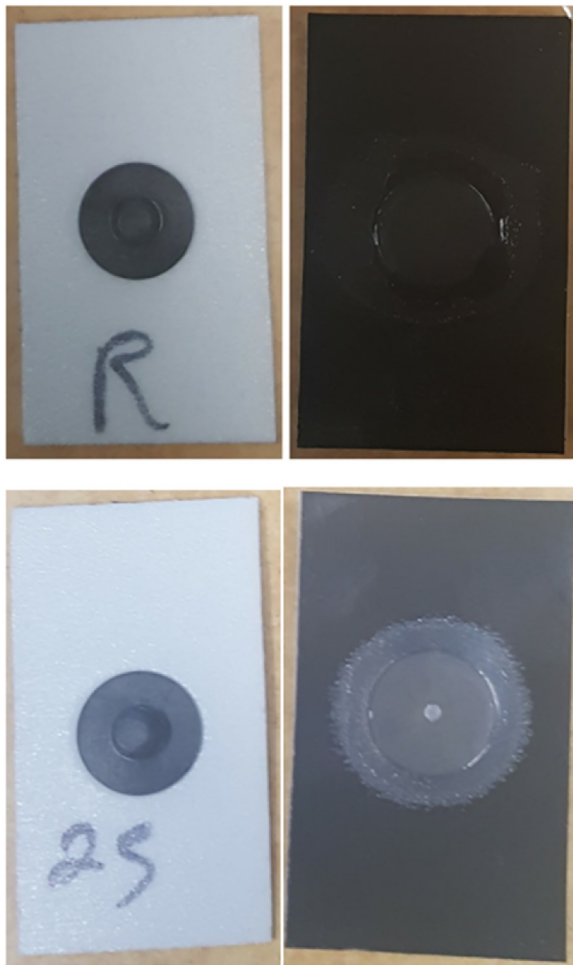
Fig. 1. Connector and contact side of tested sEMG electrodes. Top: CSA electrodes (the label R in the plot means “Reference”); bottom: SA electrodes (25% salt). Dimensions are 1 1/2” x 7/8” (3.81 cm x 2.22 cm) for both.
